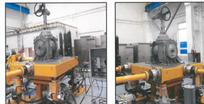
Figures 1, 2, 3, 4: EUT on test stand (Fig. 1 – test axis orientation)
