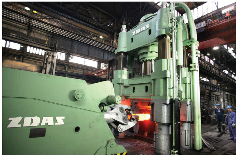
Forging Unit with CKV 1250/1600 Press and QKK 8 Manipulator, produced by ŽDAS
