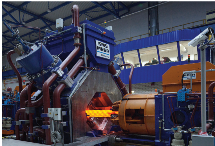
Radial Forging Machine in VÍTKOVICE MACHINERY GROUP.
