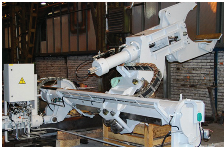
Stacking device for coil of wire, produced by Strojírny a stavby Třinec, a.s.
