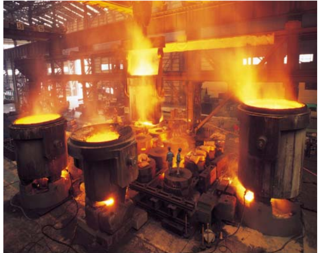
(2) Electric Arc Furnace (1) Vacuum Ladle Refining & Holding Furnace (1) Vacuum Stream Degassing Equipment
